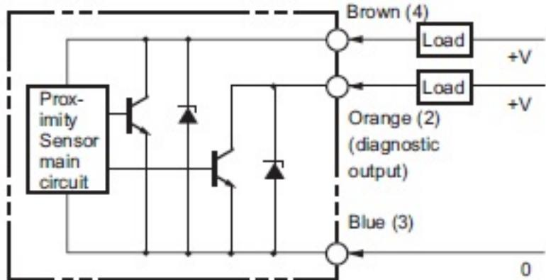
Note: Connect both the loads to the +V side of the control output and diagnostic output.
