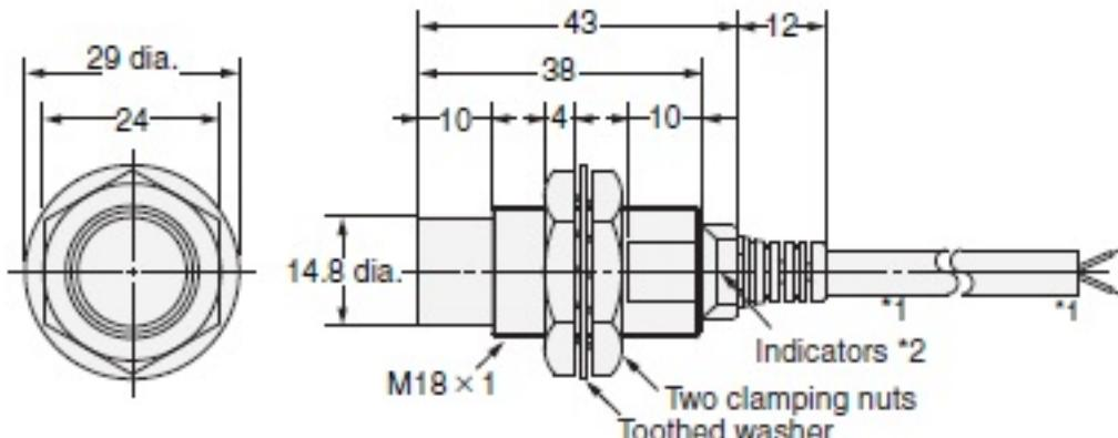
\*1. 6-dia. vinyl-insulated round cable with 2 conductors (Conductor cross section: 0.5 mm<sup>2</sup>, Insulator diameter: 1.9 mm), Standard length: 2 m
