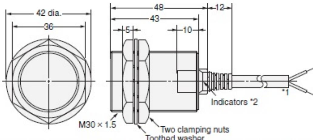
\*1. 6-dia. vinyl-insulated round cable with 2 conductors (Conductor cross section: 0.5 mm<sup>2</sup>, Insulator diameter: 1.9 mm), Standard length: 2 m
