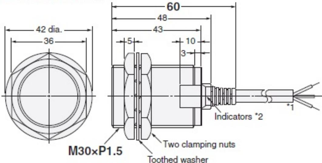
\*1. 6-dia. vinyl-insulated round cable with 3 conductors
