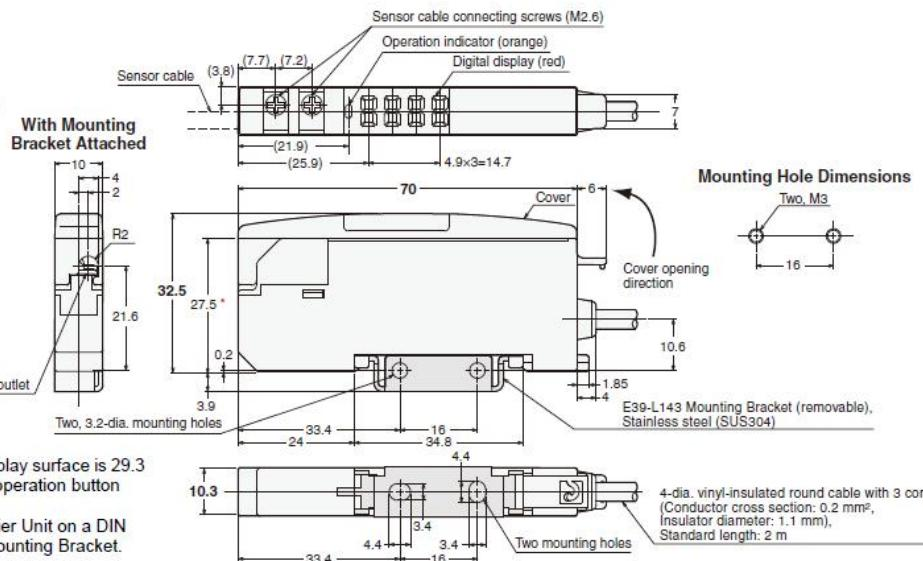
\* The dimension to the digital display surface is 29.3 mm, and the dimension to the operation button surface is 29.8 mm.
