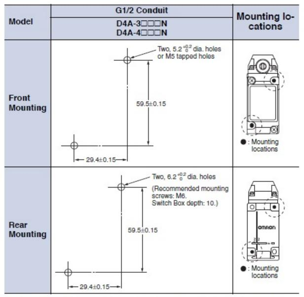
Note: For 1/2-14NPT conduits, use Two, No.10-32UNF (depth: 10) backmounting screws.
