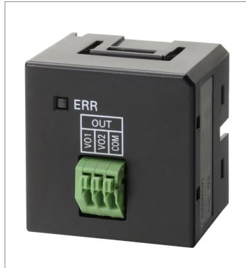
Analog Output Optional Boards CP1W-DAB21V
