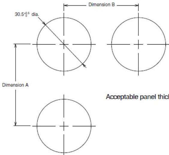
Acceptable panel thickness is between 0.8 and 7 mm.
