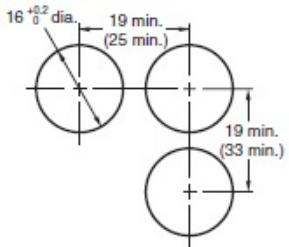
Note: 1. Make sure the thickness of the mounting panel is 0.5 to 3.2 mm.
