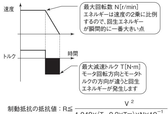
$$\text{制動抵抗の抵抗値} : R \leq \frac{V^2}{1.048 \times (T - 0.2 \times T_m) \times N \times 10^{-1}}$$
