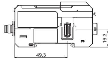
Unit coupling connector position
