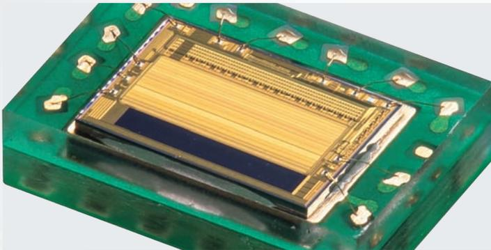
In developing ZP-L, OMRON took a deep dive into the internal structure and production process of CMOS image sensors to custom-develop high-speed, high-sensitivity, low-noise CMOS image sensors that maximize performance.
