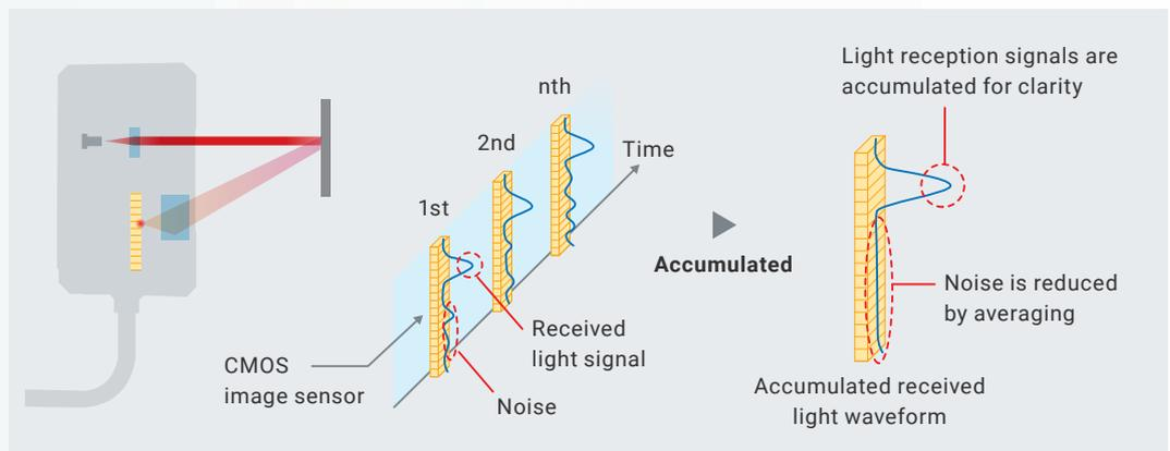
ZP-L delivers significantly higher sensitivity compared to previous products, through its unique process of integrating received light waveforms. This process amplifies the slightest light, allowing for stable detection even when the head is installed in a tilted position.
