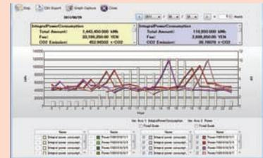
It allows past data to be displayed side by side for comparison. For example, you can display electric power of a different month on a daily basis for comparison.
