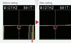
Lost part on a profile due to insufficient amount of light received
