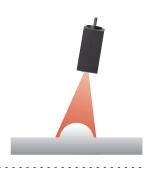
\* When inclination is great, a measurement error may occur. Check the measurement accuracy in actual measurement conditions prior to use
