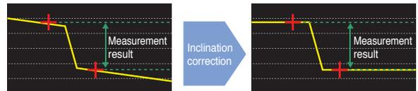
When a target is inclined, step measurement result is greater than the actual value.
