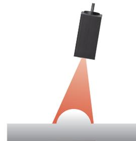
\* When inclination is great, a measurement error may occur. Check the measurement accuracy in actual measurement conditions prior to use.
