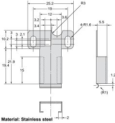
Applicable Photomicrosensors EE-SX67 $\square$  (A,P,R) (Connector Models only), EE-SX47 $\square$ , EE-SY67 $\square$ , EE-SPY31 $\square$ /41 $\square$ , EE-SPX303N/403N, EE-SPW311/411
