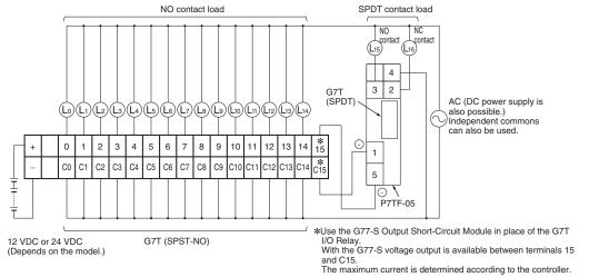
Note: If more than one G77-S Output Short-Circuit Module is employed, the voltage output of the terminals on the P7TF is as follows: P7TF-OS16: The positive side (the lower row) connects to the common line internally.
