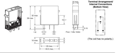
Sockets (Can be used for G7T models with SPST-NO, SPST-NC, or SPDT specifications or G3TA models.)
