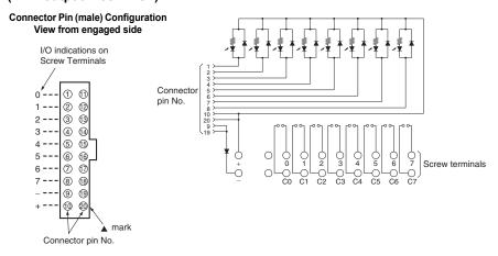
Note: Pin numbers are indicated for convenience. The ▲ mark can be used to determine orientation.
