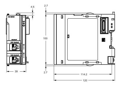
For dimensions after attaching the communications cables, refer to NX-series EtherNet/IP<sup>TM</sup> Unit User's Manual (W627).
