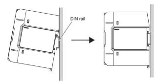
4. Raise the DIN hook and fix the body to the DIN rail
