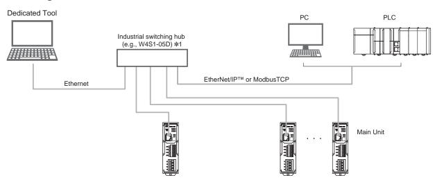
\*1. When configuring the IP address setting for main unit.
