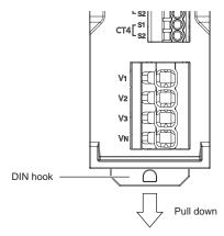
Fit the flanges of the body onto the DIN rail as shown in the below diagram, and click into place
