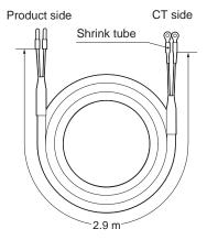
Note: The CT-supplied cable is attached to the CT.
