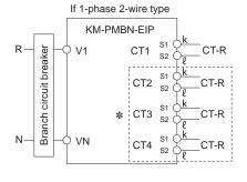
\* Wire only during multiple circuit measurements.
