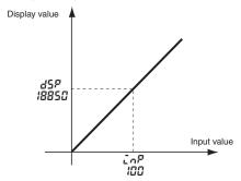
When displaying a flowrate (e.g., in  $\ell$ /min or  $\ell$ /h), make the scaling settings after confirming the I/O characteristics of the flowrate sensor. There are flowrate sensors that output analog signals. If this kind of flowrate sensor is used, consider using the K3MA-J.
