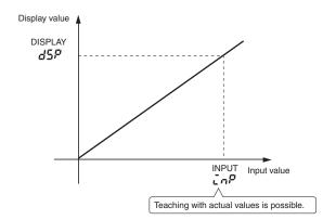
Instead of setting by inputting with the D Up Key and D Shift Key, current values can be input as scaling input values for teaching. This is useful for making settings while checking the operation status of the K3MA-F.
