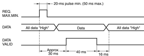
The data is set in approximately 30 ms from the rising edge of the REQUEST signal and the DATA VALID signal is output.
