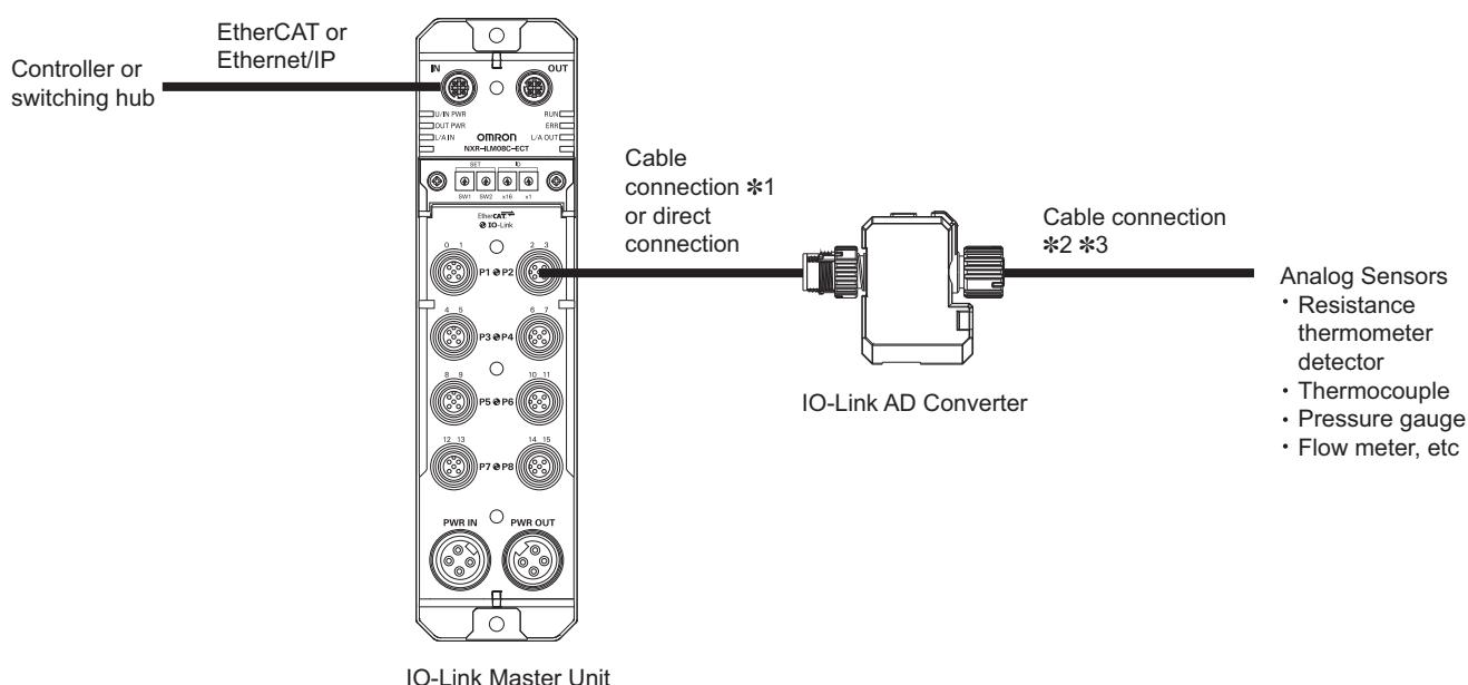
\*1. Recommended cables wiring between IO-Link master units and AD converters
