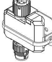
Mounting screws are not included in the package. The mounting screws (M3, minimum length 3 mm, screw head height including washer 4 mm or less) are recommended.
