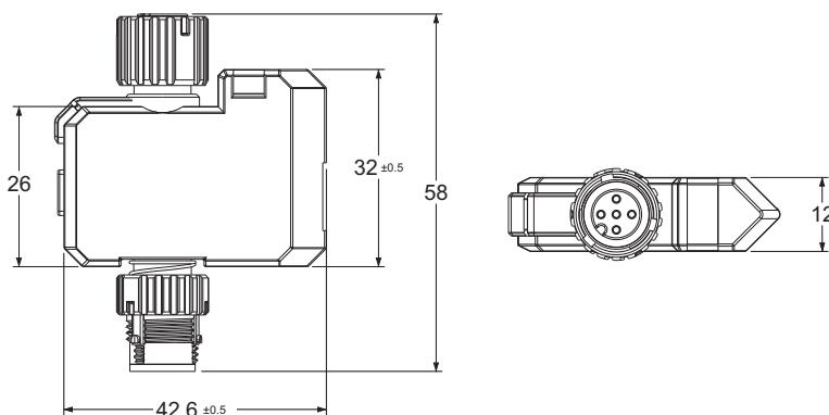
Dimensions when some K3CVs connect directly to the NXR.
