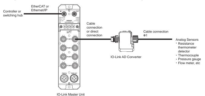
\*1. For the thermocouple input types, be sure to use compensation wires. Otherwise, this may cause a temperature error. Refer to page 3 for selection of connectors and compensation conductors.
