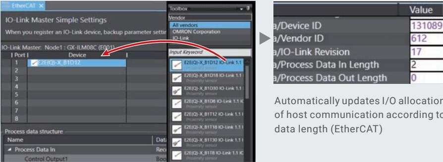
The screenshot shows the 'IO-Link Master Simple Settings' window in Sysmac Studio. On the left, a table lists IO-Link devices connected to Port 1. A red arrow points from the 'E2E(Q)-X\_B1D12' device in this table to the 'Input Keyword' list in the 'Toolbox' on the right. Another red arrow points from the 'E2E(Q)-X\_B1D12 IO-Link 1.1' keyword to a parameter table on the right.
