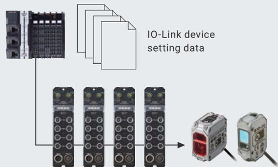
Configuring all devices at once from the controller eliminates the need to configure each device individually, greatly cutting down setup time and effort.
