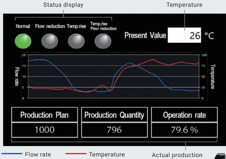
Simultaneously monitoring the flow rate and temperature of cooling water enables cooling to be maintained and controlled. This ensures a consistent finish and raises the standard of parts strength.
