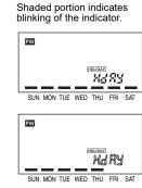
3. Press WRITE to enter the setting. After "HdRY" is displayed for approximately 1 s, the Time Switch returns to RUN mode.
