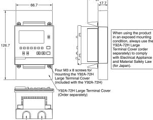
Y92F-90 DIN Track Mounting Base (Order separately) DIN Track Mounting panel ΉE 71.1 \*1 79.8 \*2 Using a PFP-50N or PFP-100N Note: 1. Osing a FTP-correction of the correction of the corre
