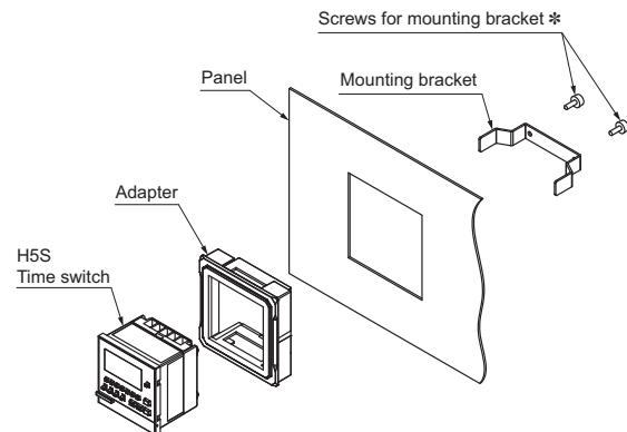
\* These screws are included with H5S-□A□/-□B□ Flush Mounting Models.
