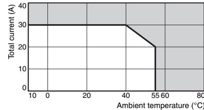
If wires with a temperature rating of 105 °C or higher are used, refer to the derating curve in *Specifications* on page 3.
