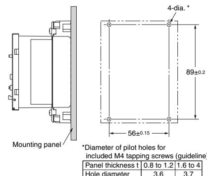
\*Diameter of pilot holes for included M4 tapping screws (guideline)
