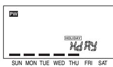
3. Press [WRITE] to enter the setting. After "HdRY" is displayed for approximately 1 s, the Time Switch returns to RUN mode.
