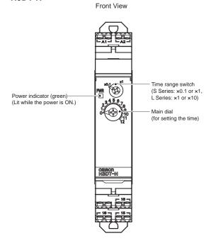
Note: If the switch is left between settings, proper operation may not be possible. Make sure that the switch is set properly.
