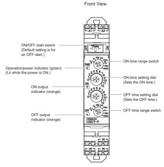
Note: If the switch is left between settings, proper operation may not be possible. Make sure that the switch is set properly.
