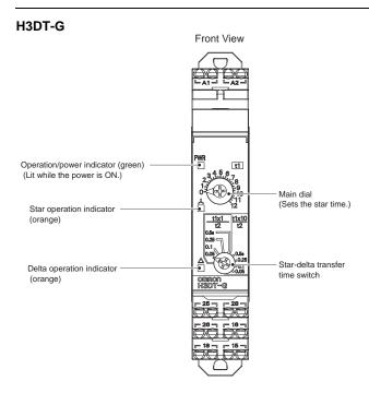
Note: If the switch is left between settings, proper operation may not be possible. Make sure that the switch is set properly.
