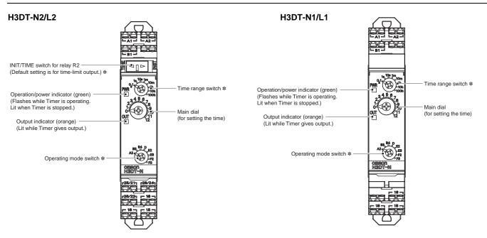
\* If the switch is left between settings, proper operation may not be possible. Make sure that the switch is set properly. Note: The default settings are for 0.1 s in mode A2 for the H3DT-N and mode A for the H3DT-L.
