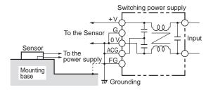
Insert a plastic insulator of approximately 10 mm between the Sensor and the mounting base.
