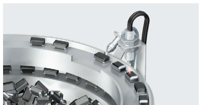
Air blower output during chip's front/rear detection
