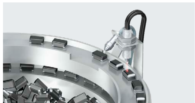
Air blower output during chip's front/rear detection
