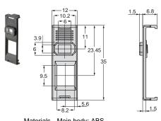
Main body: ABS Lens: Methacrylic resin (PMMA)
