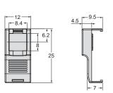
Main body: ABS Materials Lens: Methacrylic resin (PMMA)
