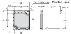
Materials Reflective surface: Methacrylic resin (PMMA) Back surface: Polybutylene terephthalate (PBT)
