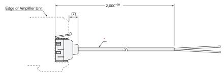
\*4-dia. cable with 2 conductors, Standard cable length: 2 m (Conductor cross-section: 0.2 mm² (AWG24), Insulation diameter: 1.1 mm)
