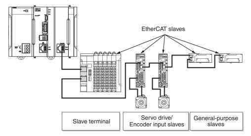
EtherCAT is synchronized with the servo cycle of the CK $\square$ M-series CPU Unit. This enables acquisition of the I/O data of slave terminals that are synchronized with the servo cycle.
