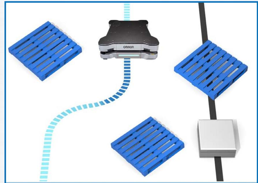
Unlike autonomous mobile robots (AMRs), automated guided vehicles (AGVs) require guides, which restricts their options for routing.
