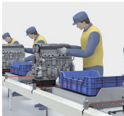
Presence detection of pallets
